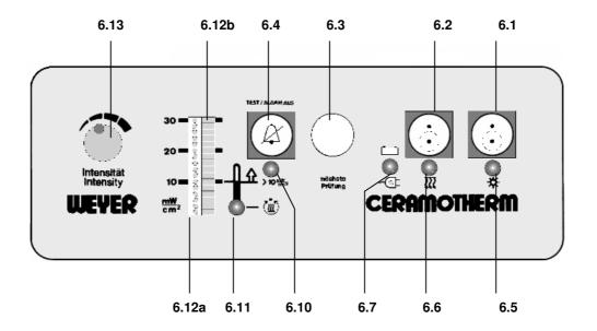
In order to start the extended functional test, the device must be warmed-up to a value above 10 mW/cm<sup>2</sup>. Select an intensity of 12 mW/cm<sup>2</sup> with knob (6.13) and wait until this value is reached. The LED (6.12a) and the bar graph 6.(12b) must indicate the same value.
