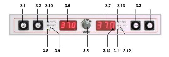
Warm-up the under-pad heating to a temperature between 35°C and 37°C, until warning lamp (3.12) extinguishes.
