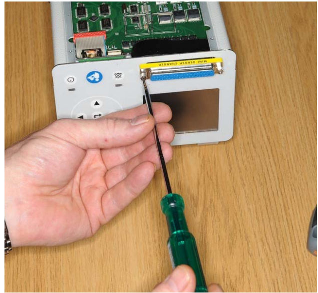
4. Remove the connector saver
