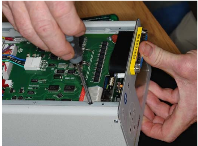
2. Mount the display assembly. Fit the connector saver, adjust then the position and tighten the four main board screws.
