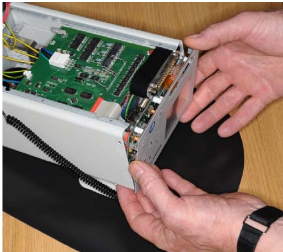
5. Carefully loosen the display assembly from the cabinet
