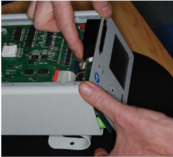
1. Slide the display assembly carefully in under the plastic protective sleeve.
