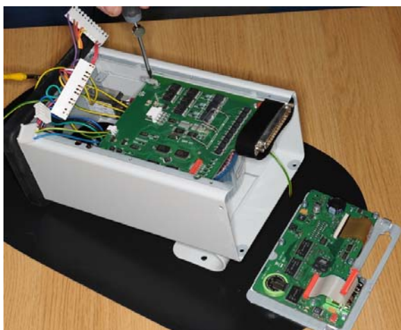
7. Loosen the 4 main board screws
