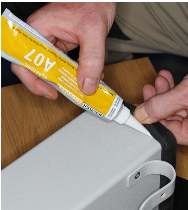
3. Mount the rubber frame. Be observant to position the cavities over the screw heads. Adjust the frame for a nice close fit. Carefully apply a small amount of Wacker Elastasil A07 under the frame - close to the corners. Remove any excessive silicone.
