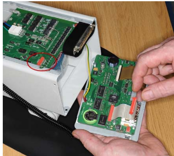
6. Remove the flat cable and the earth cable.
